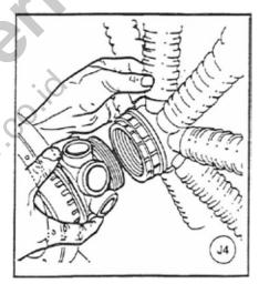
STEP 5 Hold Hub assembly with one hand and attach laterals as described in (step 3). After all laterals are assembled, bond pipe to adaptor using universal primer and cement.
