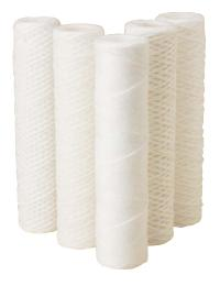
Pentair<sup>‡</sup> Pentek<sup>‡</sup> WP Series Cartridges are manufactured from a durable polypropylene string that is wound around a rigid polypropylene core. They are premium string wound solution to reduce fine sediment, including sand, silt, rust and scale particles.
